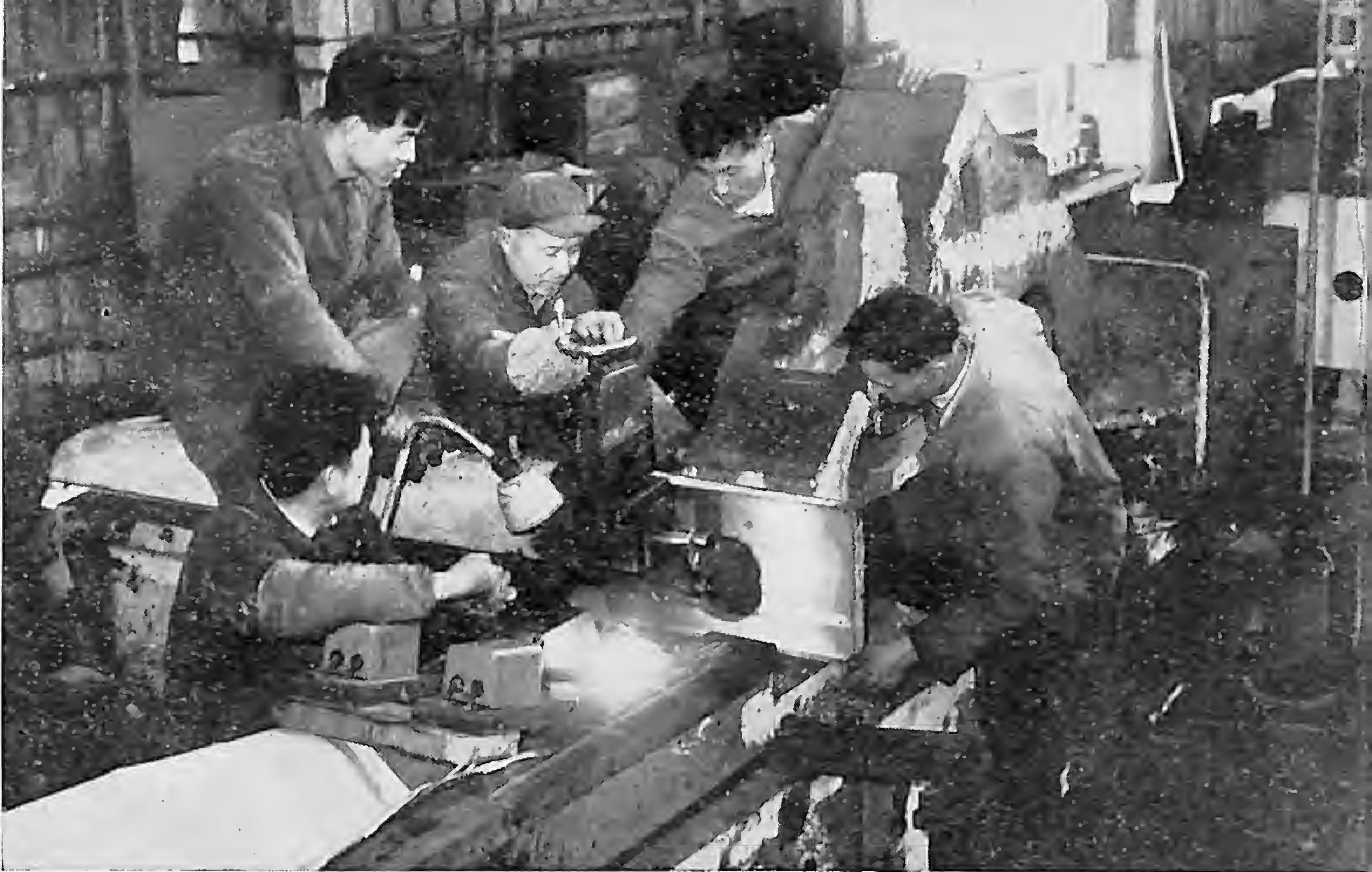
Workers and cadres at the Chiensheh Machinery Plant study the way a small shaper processes a large roll crusher.
